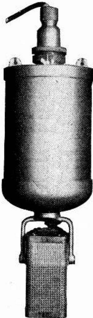
The R.C.A. Ribbon microphone consists of an electrodynamic transmitter and amplifier.
